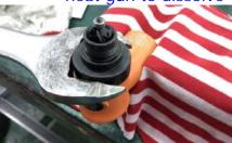
Step 10. Pull out Rotor assembly (#1 $\sim$ #9 + #18) after #13 is taken off.
