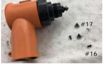
Step 9. Fix #19 Houshing with a vise and blow #13 Connect Nut with a heat gun to dissolve the glue on #13. Then, #13 can be taken off.
